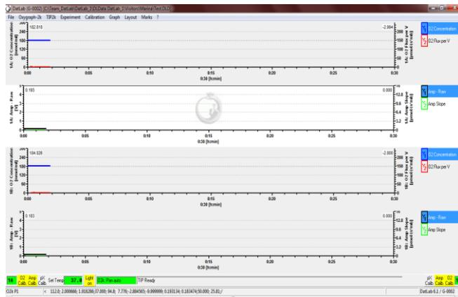
of using Saf it is appropriate to initially select the layout 'Safranin raw signal' which displays data related to respirometry according to the standard layout '05 Flux per Volume corrected' and the Saf signal as plots of the raw signal 'Amp Raw' [V] just below each related plot of the oxygen signal.
