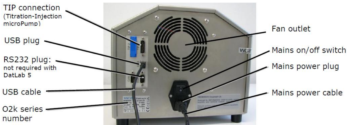
Rear of the Oxygraph-2k main unit Series E.
